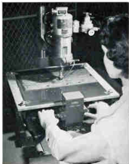
The Type 3005 PANTODRILL, a semi-automatic drilling machine designed for rapid, economical and accurate drilling of large numbers of holes in printed wiring boards.
