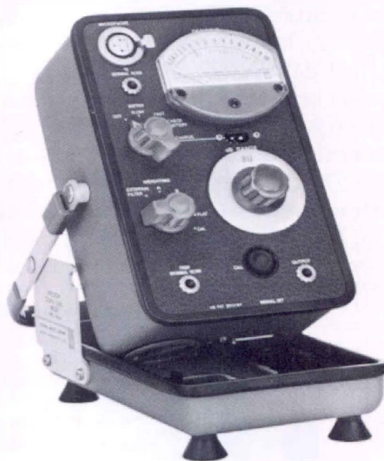
Figure 1. Precision sound-level meter, portable model.
