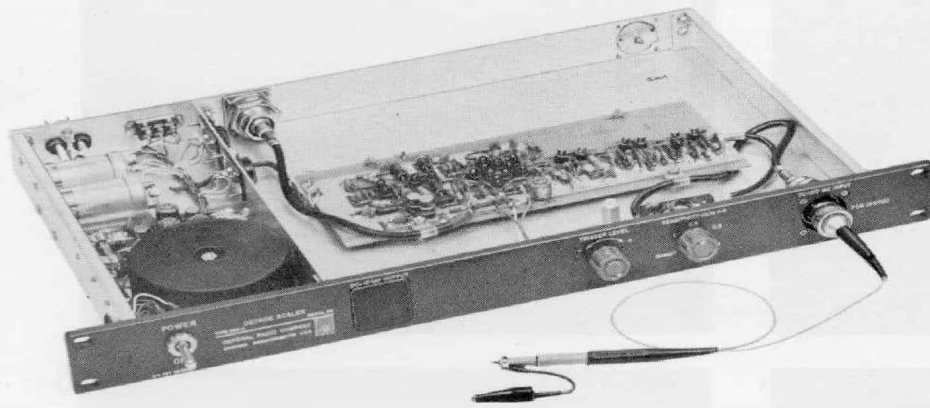
Figure 6. Tektronix oscilloscope probe (foreground) can be plugged directly into the scaler. The scaler input and output terminals can be mounted either on the panel or at the rear. Cover plates are provided for the panel when rear connections are used.
