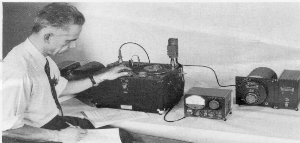
Type DNT-5 Heterodyne Detector in use with the Type 916-AL RF Bridge.
