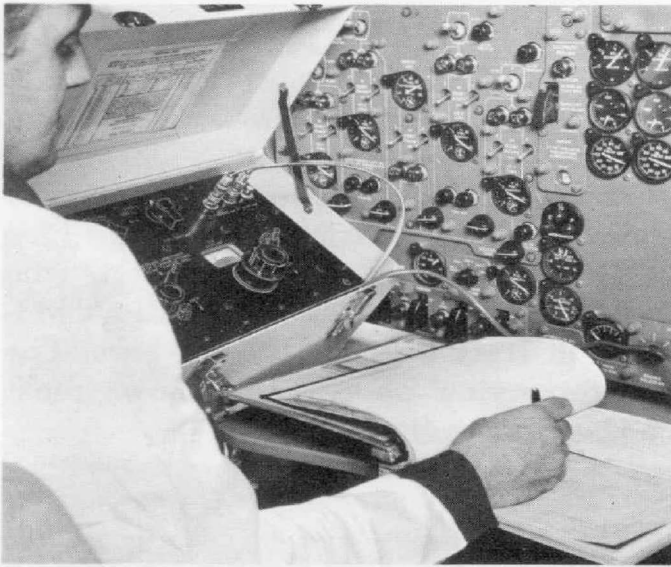
Technician calibrates fuel gage of modern jet aircraft by means of a GR Type 1429-A Fuel-Gage Tester.
