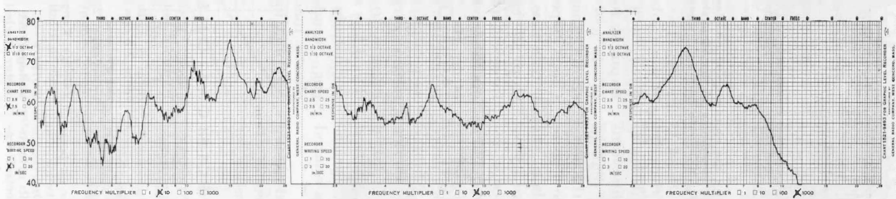
Figure 9b. Sound-pressure spectrum in the vicinity of an air compressor, measured with the recording analyzer and the Type 1560-P4 PZT Microphone Assembly.
