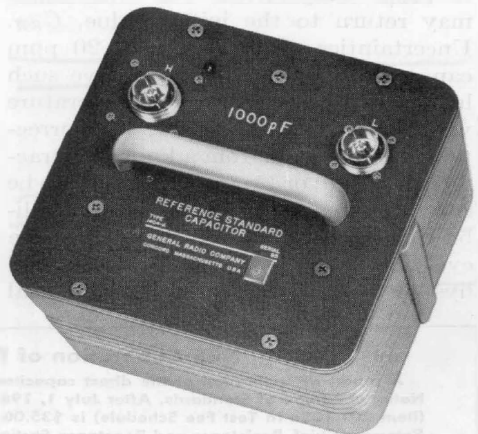
Figure 3. Panel view of the Reference Standard Capacitor.
