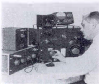
Calibrating Type 1423-A Precision Decade Capacitors in the General Radio Standardizing Laboratory using the Type 716-C Capacitance Bridge.
