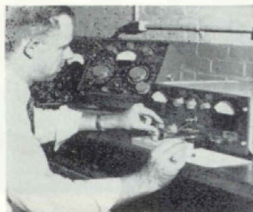
Measuring the collector-to-base capacitance of transistors with the Type 1605-A Impedance Comparator.
