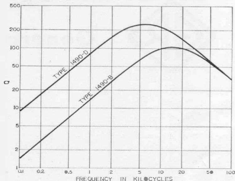
Figure 2. Plot of Q versus frequency for the 1-milli-henry step in the old and new decade inductors.
