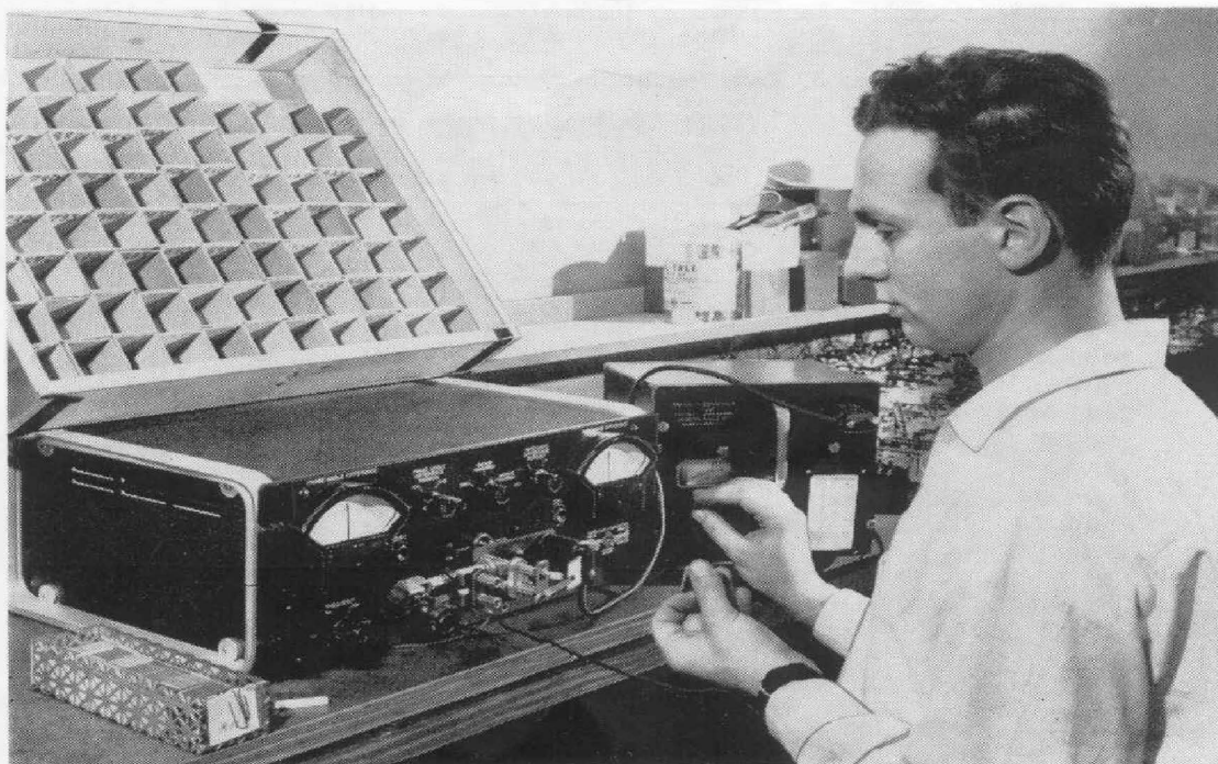
Figure 4. Mica for the Type 1409 Standard Capacitors is selected for low losses in this test setup using the Type 1605-A Impedance Comparator.
