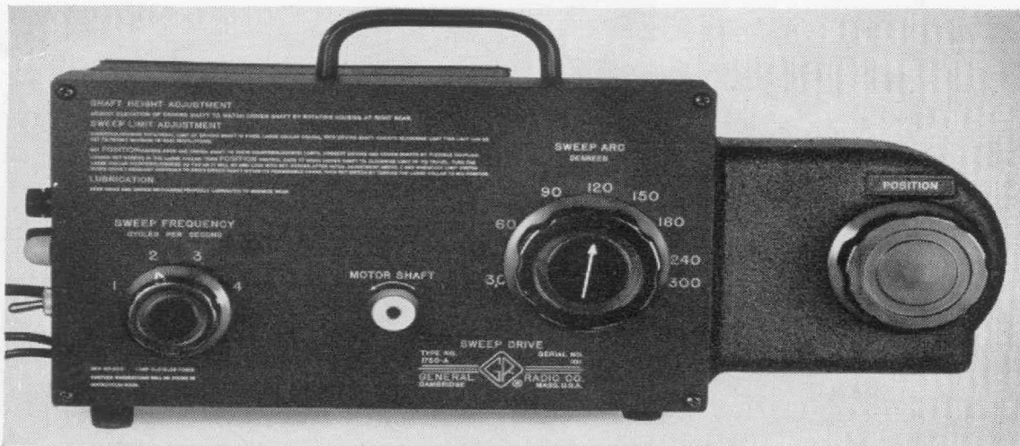
Figure 2. Front panel view of the Type 1750-A Sweep Drive, showing the SWEEP FREQUENCY, SWEEP ARC, and POSITION controls.
