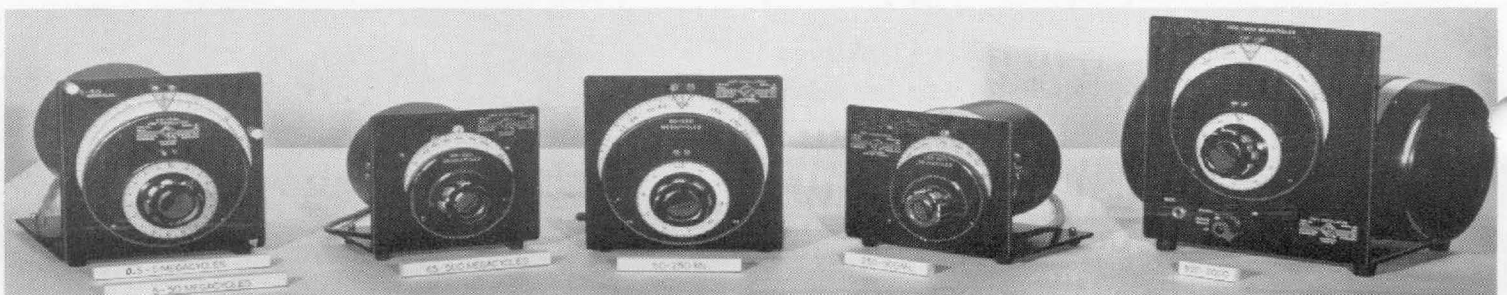
Figure 2. Group of Unit Oscillators covering a frequency range of 0.5 to 2000 megacycles. The lengths of the bars in front of the units indicate their frequency coverage on a logarithmic scale.
