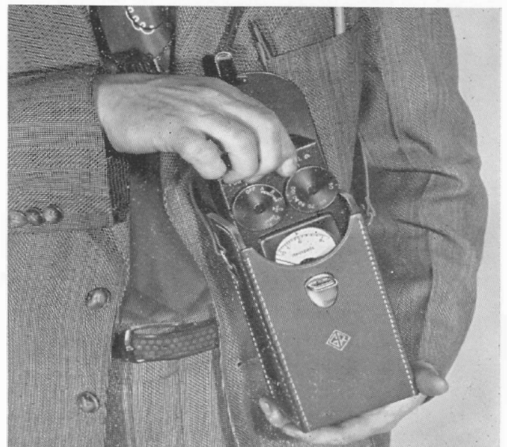
Figure 4. The Transistor Oscillator fits into the same convenient leather carrying case as the Sound-Survey Meter.
