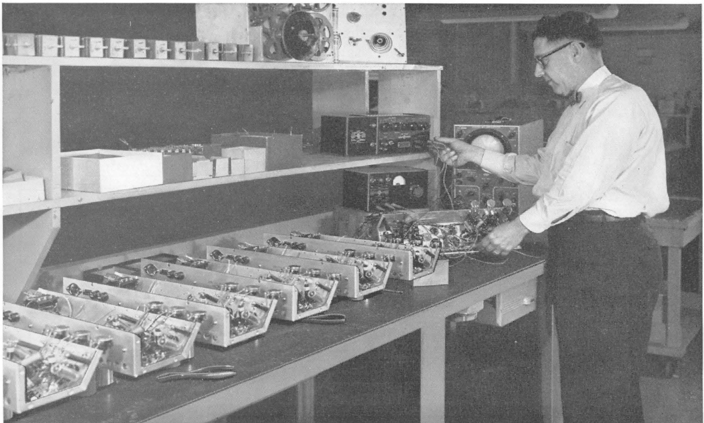
Figure 6. The Unit Pulser used for production tests on amplifier assemblies.
