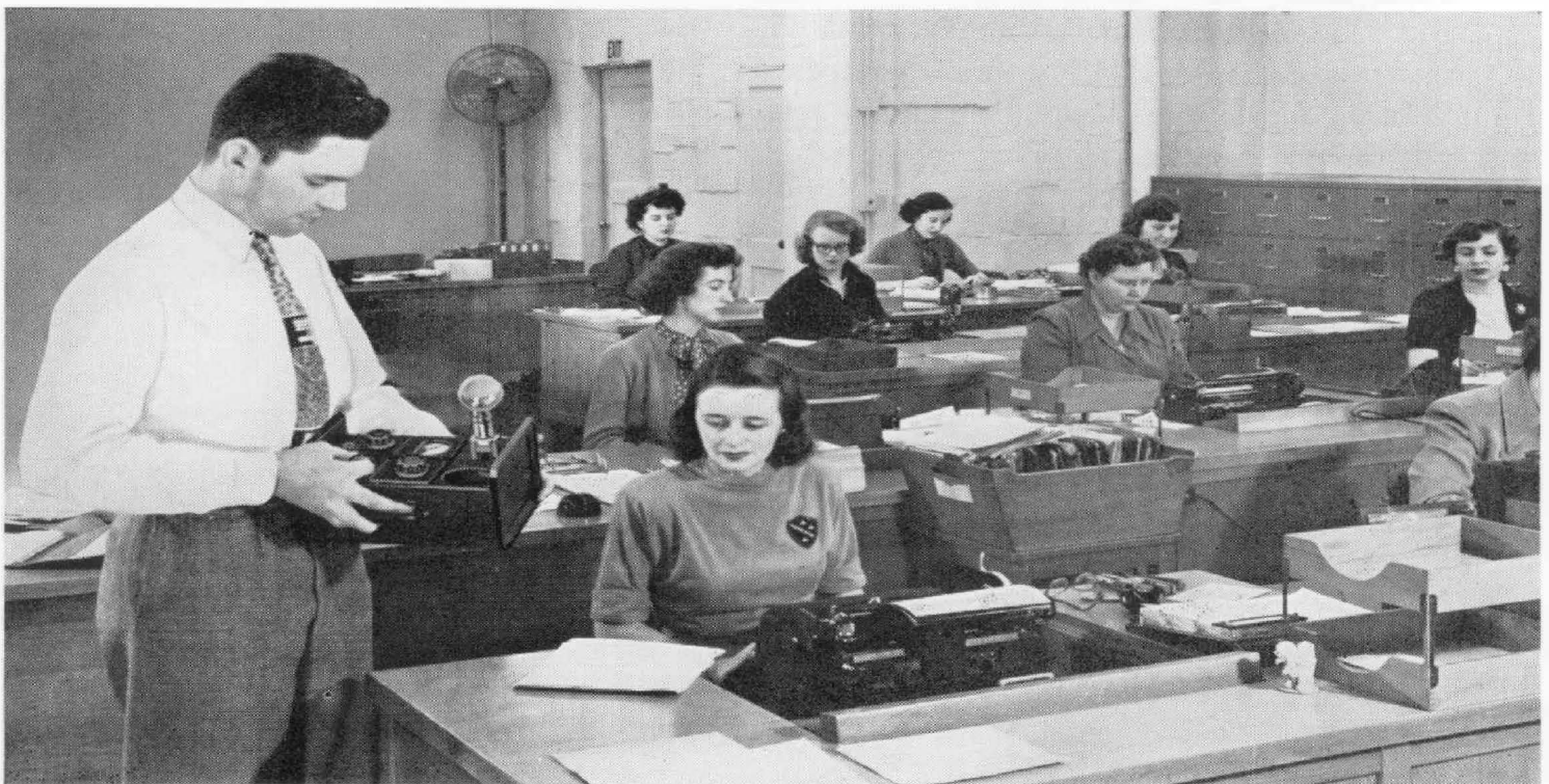
Figure 5. Determining noise level and speech-interference level in a business office with the Type 1551-A Sound-Level Meter.
