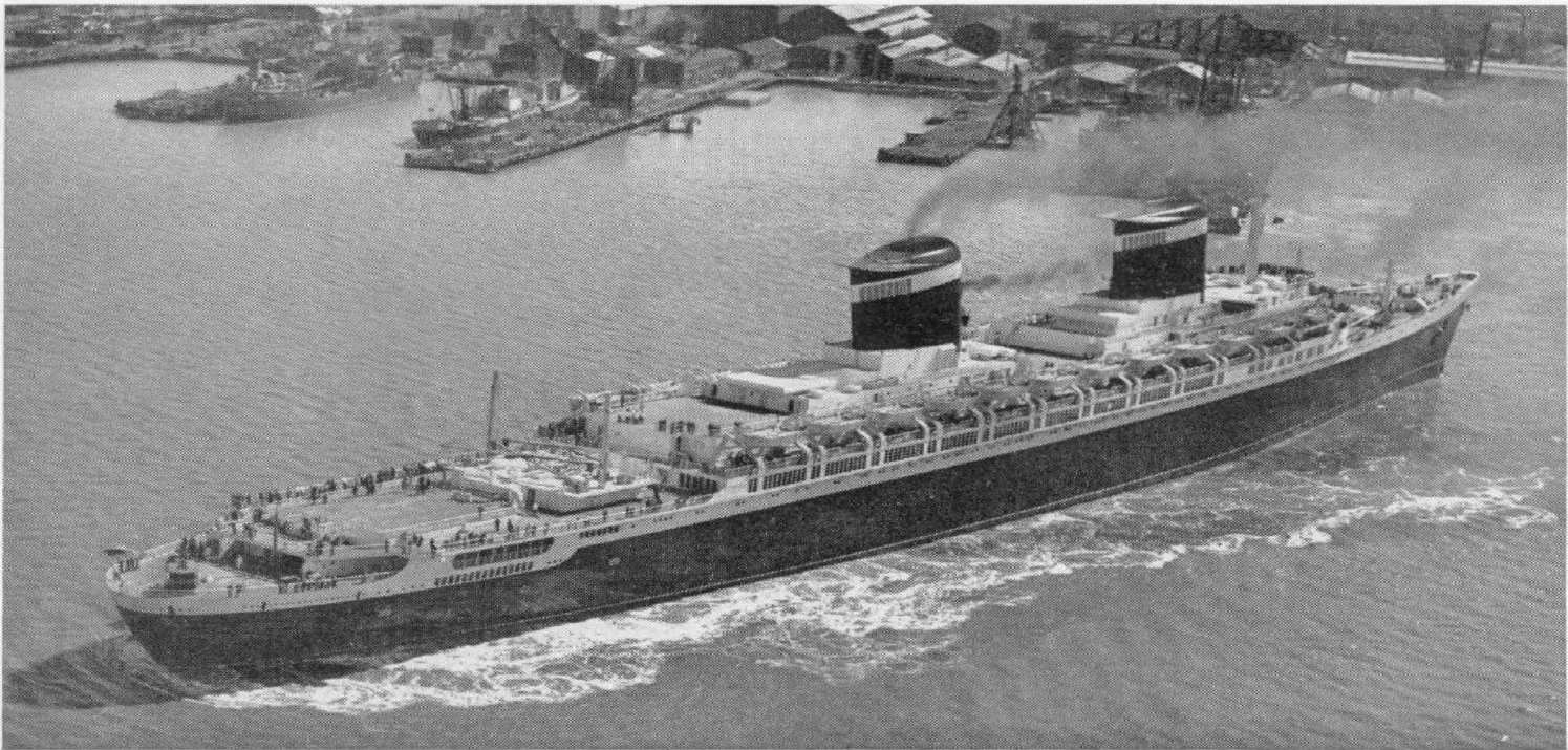
The SS United States , new holder of the Atlantic blue ribbon, has attained speeds of 35.59 knots on her east-bound voyage, 34.51 knots on her westbound voyage, and an average speed of over 35 knots in her initial voyages.
