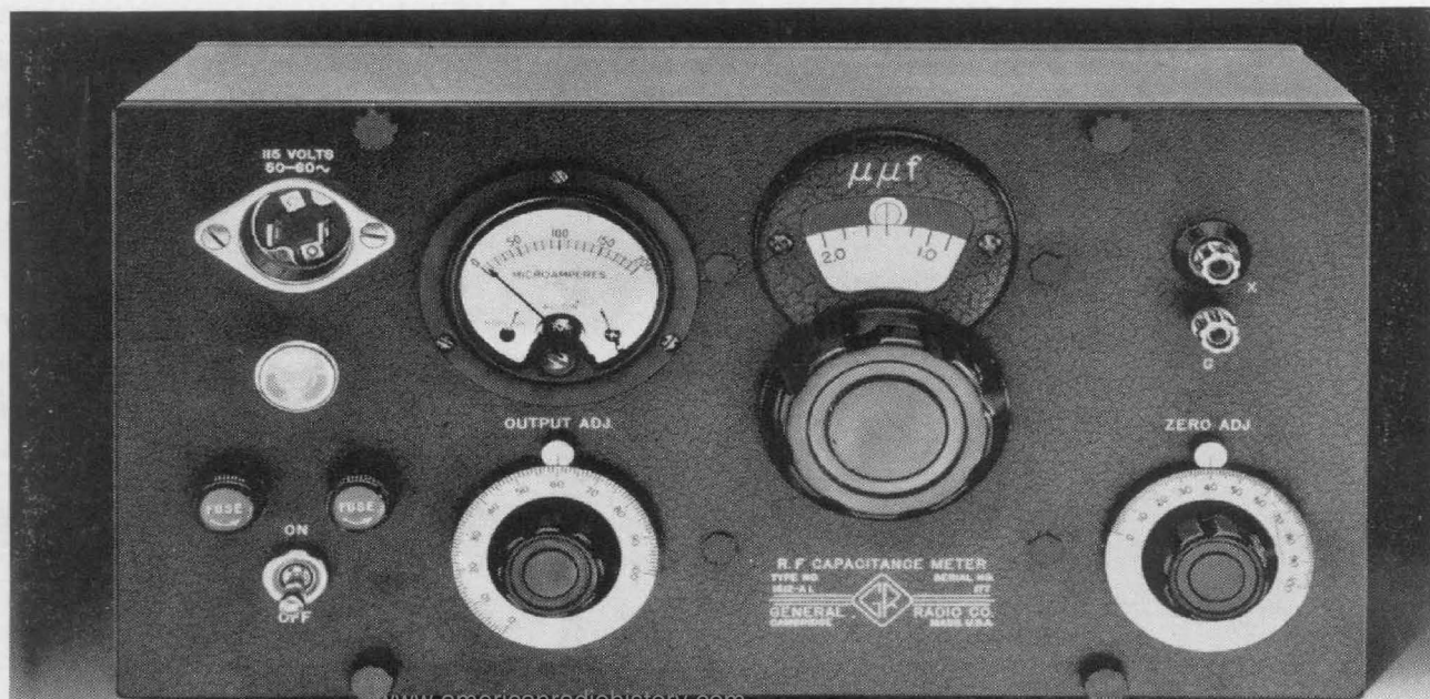
Figure 1. Panel view of the Type 1612-AL R-F Capacitance Meter, showing open capacitance scale at low end of range.
