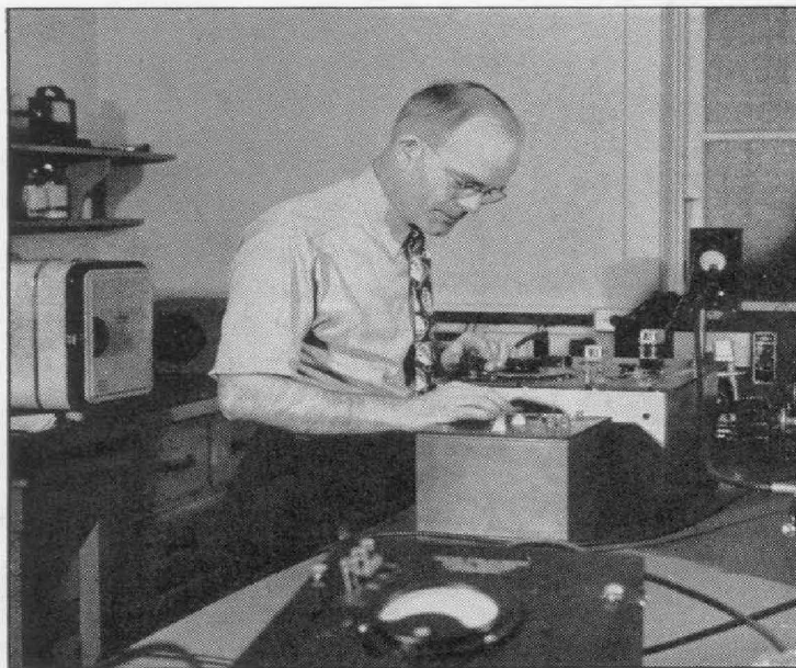
FIGURE 17. D. H. Chute, in charge of the measurements room, balances a precision capacitance bridge.
