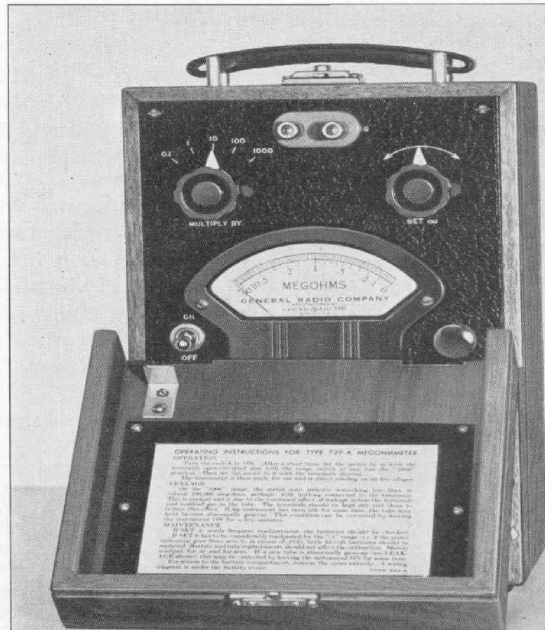
FIGURE 1. View of the TYPE 729-A Megohmmeter showing the compact portable construction. The cover, shown folded back, is removable.
