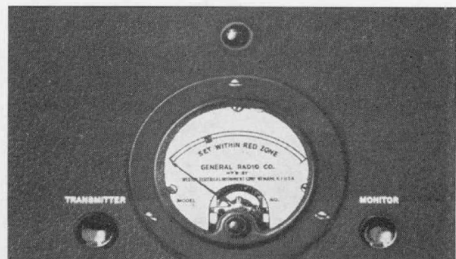
FIGURE 4. The signal-level indicator on the frequency monitor unit. When the input level is correct, the meter reading is within the red (shown black in the photograph) range on the scale.
