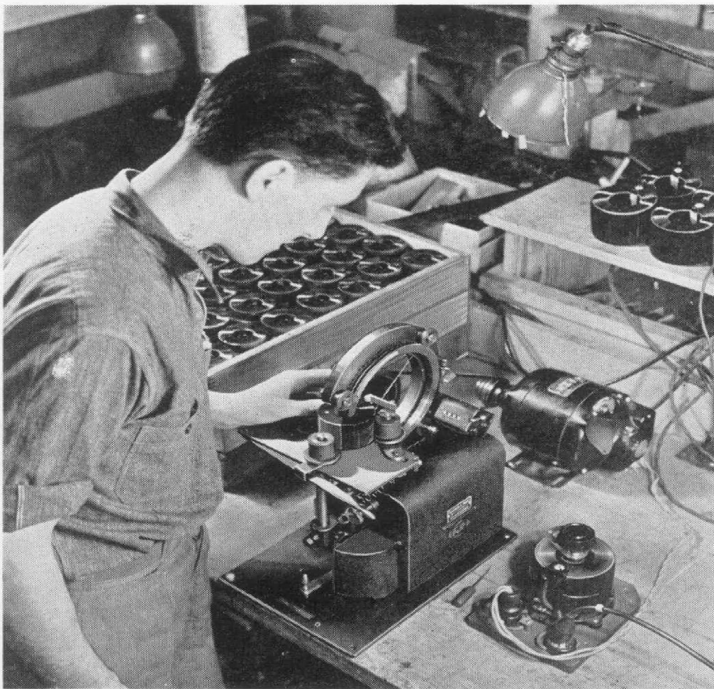
TYPE 200-B Variacs are wound on the machine shown above
