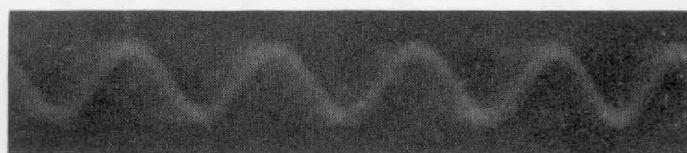
Spread-out traces from a 60-cycle voltage obtained by swinging the camera on a pivot. Fast-screen tube on the left, slow-screen tube on the right. Note the absence of blur in the fast-screen trace
