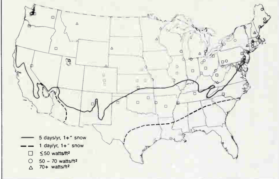
Figure 2: Selected anti-icing heat flux values
