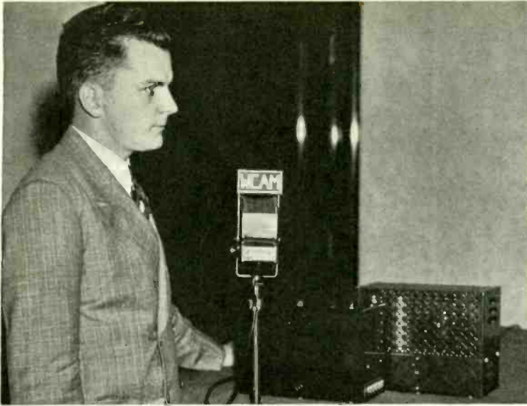
SHOWING THE AUTHOR WITH THE VELOCITY MICROPHONE, LINE AMPLIFIER, AND POWER-SUPPLY TESTED AT W.C.A.M.
