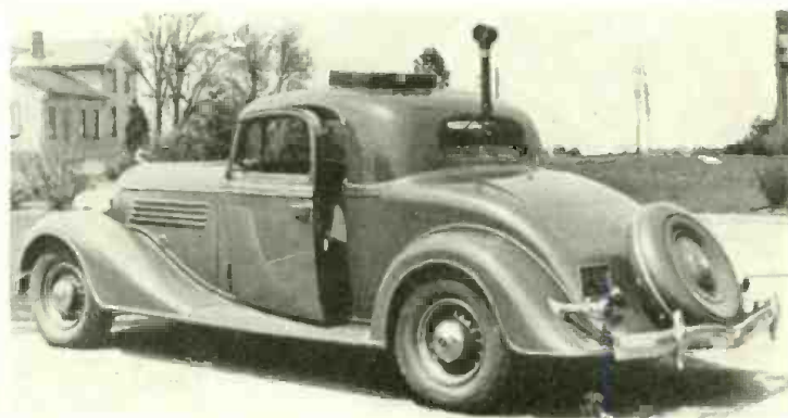
FIG. 2. SHOWING THE LOOP FIXTURE EXTENDED THROUGH THE REAR WINDOW OF THE CAR.
