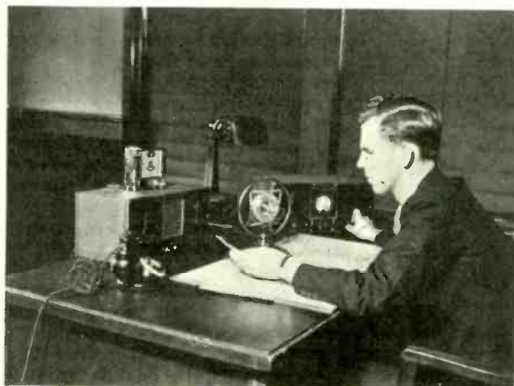
OPERATOR HARPER AT THE CONTROL DESK. SHOWN IS THE RECENTLY INSTALLED WESTERN ELECTRIC 89-A SPEECH AMPLIFIER AT THE RIGHT. THE 19-A STATION RECEIVER IS SHOWN AT THE LEFT AND THE 600-A MICROPHONE IN CENTER.
