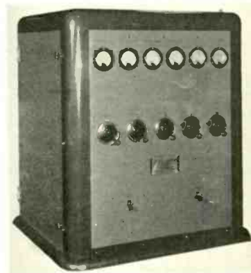
FIG. 3. ET-5017 ULTRA-HIGH-FREQUENCY TRANSMITTER, 25 WATTS, CRYSTAL CONTROL, 30-41 MEGACYCLES.
