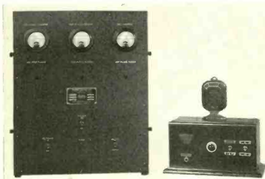
FIG. 2. ET-5004 ULTRA-HIGH-FREQUENCY TRANSMITTER, 30-36 MEGACYCLES, 15 WATTS, MASTER OSCILLATOR, POWER AMPLIFIER TYPE.
