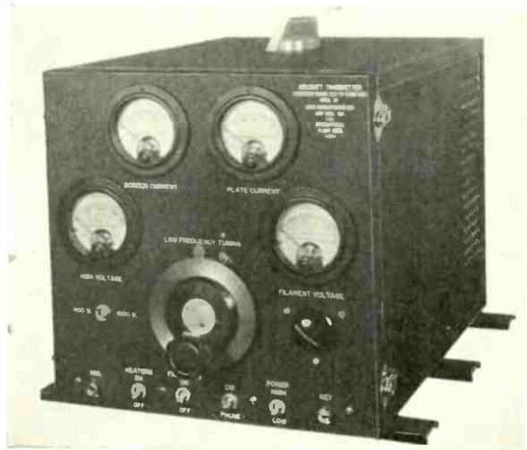
FIG. 1. Front view of the 9-band transmitter which has a frequency range of 300 to 17,000 kc. There are eight crystal-controlled frequency bands and one self-controlled frequency band, tuning for the latter being controlled by the precision dial on the front panel. Note wave-changing control knob on top of the case.
