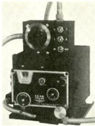
Fig. 6. The aircraft beacon receiver which tunes from 195 to 415 kc, through the airway beacon channels. Upper part of receiver shows a special loop tuning unit which does not ordinarily accompany this set.
