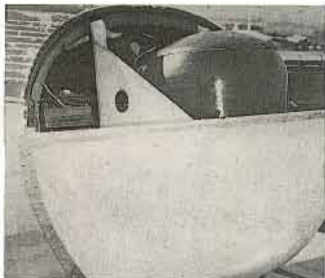
Closeup of radar and radome used in Southwest Airways plane. The rear of the indicator unit comes to within 8" of its transmitter-receiver.
