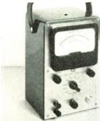
Above: A portable tone generator, for use in equalizing remote telephone lines, which features an RC type circuit allowing selection of ten frequencies from 50 to 15,000 cps. Below: Portable remote three-channel amplifier using type 1620 indirectly heated tubes. Each channel is said to offer an overall gain of 92.5 db. (Courtesy RCA)
