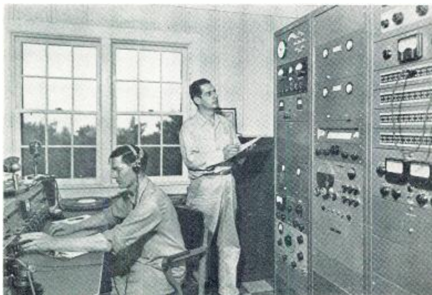
Operating room of one of the network stations. Equipment and layouts at all of the stations are identical. Apparatus in top panel in the left hand rack is used for the collection of weather information.
