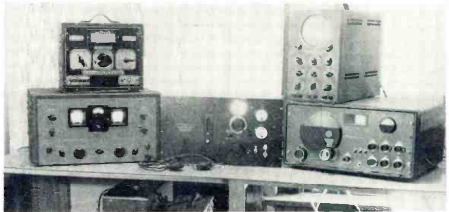
Figure 5 Setup for frequency measurements using the standard and two receivers.
