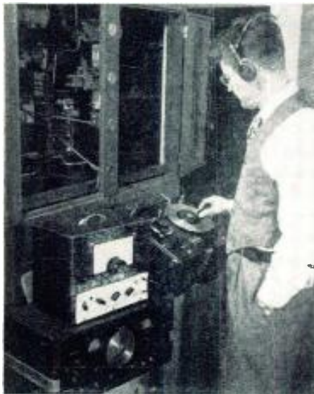
Author measuring impedances in a 5-kw Doherty amplifier with an r-l bridge, signal generator, and detector-receiver.
