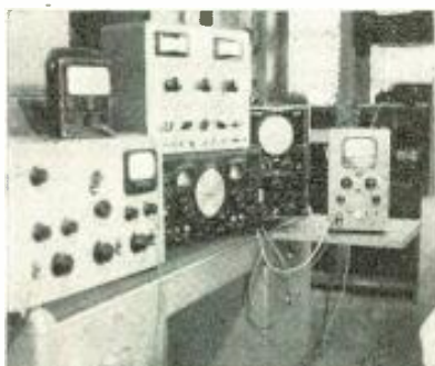
Setup for testing a receiver. Left to right: test set, signal generator, distortion noise analyzer, communications receiver, 'scope and vtvm.
