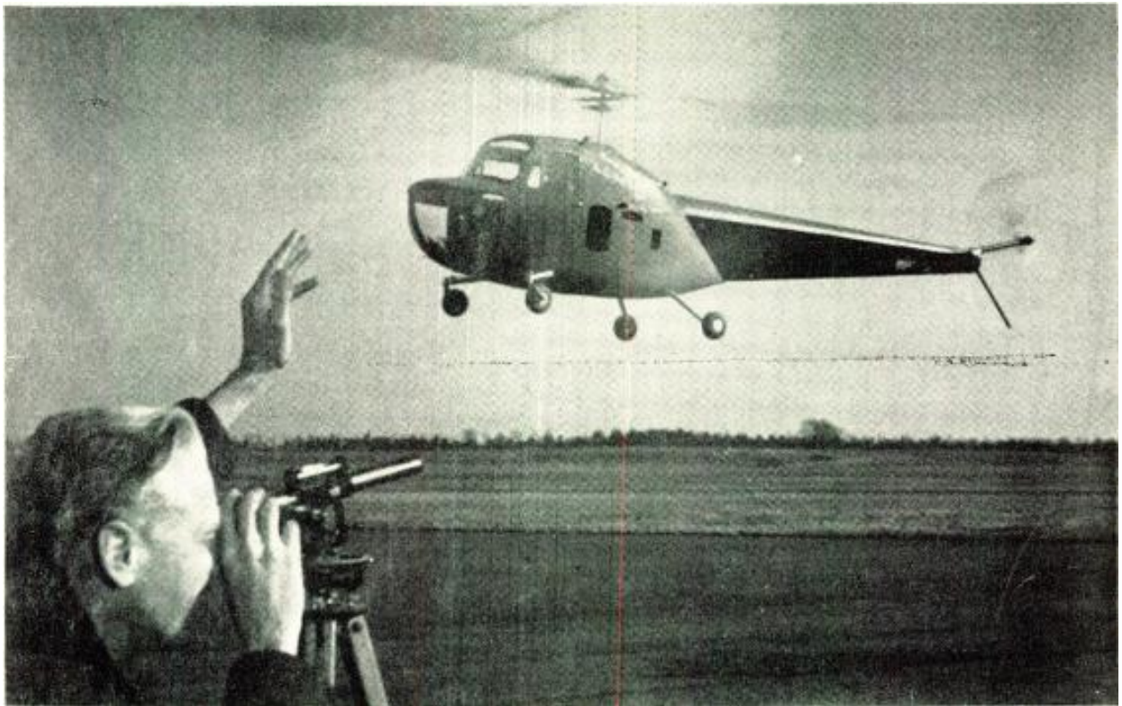
H. R. Skifter guiding a helicopter into position over the reference point to take measurements of the vertical component of a broadcast station's output.
