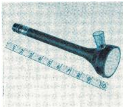
The 2½" magnetic-deflection picture tube, with a base picture size of 1.4" x 1.86".
