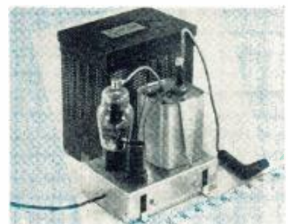
High voltage 25-kv power supply designed as second-anode power supply.
