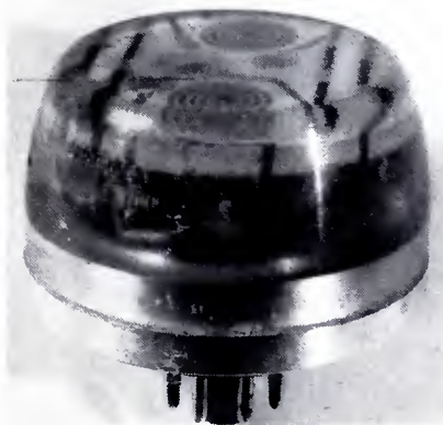
Above: Cast resin plug-in p-c unit. The unit contains a complete amplifier with sub-miniature tubes. (National Bureau of Standards).
