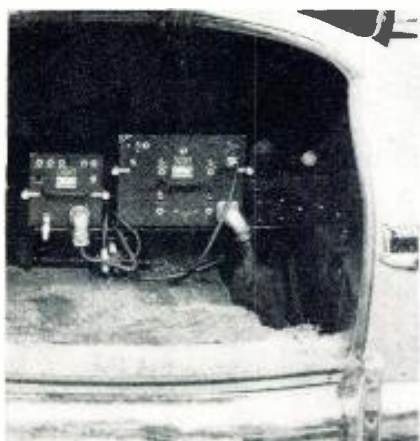
The receiver (left), transmitter (right) and power supply in trunk compartment of taxicab.
