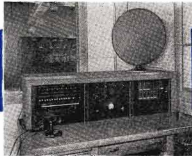
1926. The first coordinated speech input system was this Western Electric 7A, with all controls in a wooden console mounted on a desk. First to use rectified a-c for plate supply.
