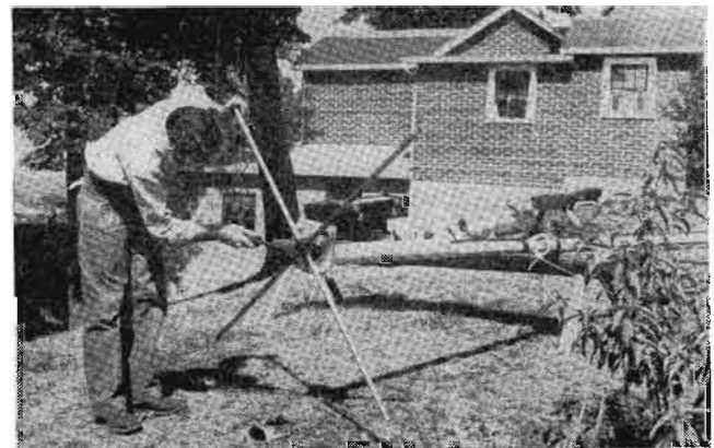
Figure 4 Mr. Yazell applying the finishing touches to the temporary 101.1-mc antenna, a composite turnstile. Temporary studios of WCFC are in building at rear.
