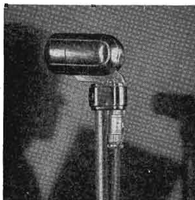
Turner "211" Mike with steel shell "XL" plug. Special adapters are required to re-convert these mike receptacles to "XL".
