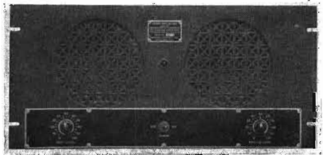
Figure 11. Front view of the speaker amplifier unit. Two 6" p-m speakers are used. Controls permit adjustment of the input level and the monitor line level. Figure 12. Rear view of the speaker amplifier unit showing the two speakers, power supply, input and output components and terminal strip.
