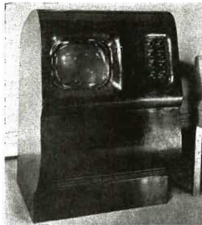
Figure 14 Direct-viewing color television receiver developed by CBS. Uses a 10" tube with view magnified to approximately the size of a 12" tube.
