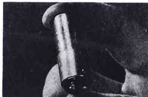
Miniature cold cathode voltage regulators, 1 1/4" x 3/4", for 65 to 90-volt operation where currents range between 2 and 3 milliamperes and maximum voltage variation may not exceed 3 volts, developed by Sylvania.
