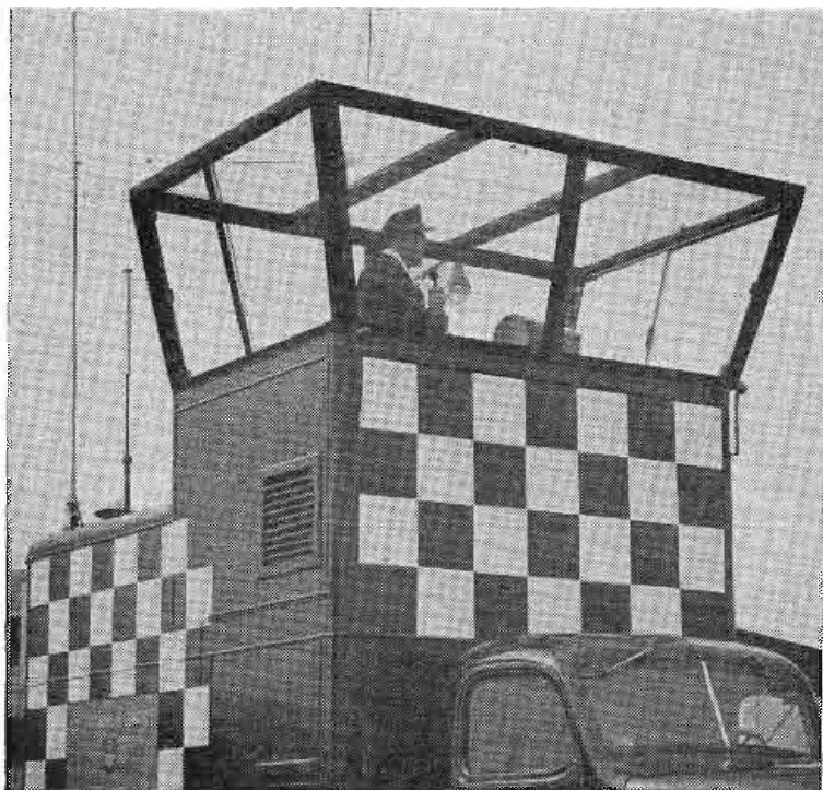
Left, mobile airport traffic control tower developed by the air traffic control division of the CAA in collaboration with the Engineering and Signals Division of the Army. Operated by two men. Incorporates a power plant capable of producing 5,000 volts for the operation of six intermediate frequency receivers, four u-h-f receivers, a low frequency transmitter and an u-h-f transmitter. Right, portable experimental u-h-f localizer.
