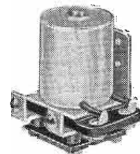
SERIES SC-5 SOLENOID CONTACTOR. Contacts rated at 75 amps. continuous, 300 amps. surge. Contact combination—single pole single or double throw. Coil operates on 18-28 volts D. C. and consumes 7 watts at 24 volts D.C. continuous. Send for bulletin SC-5.
