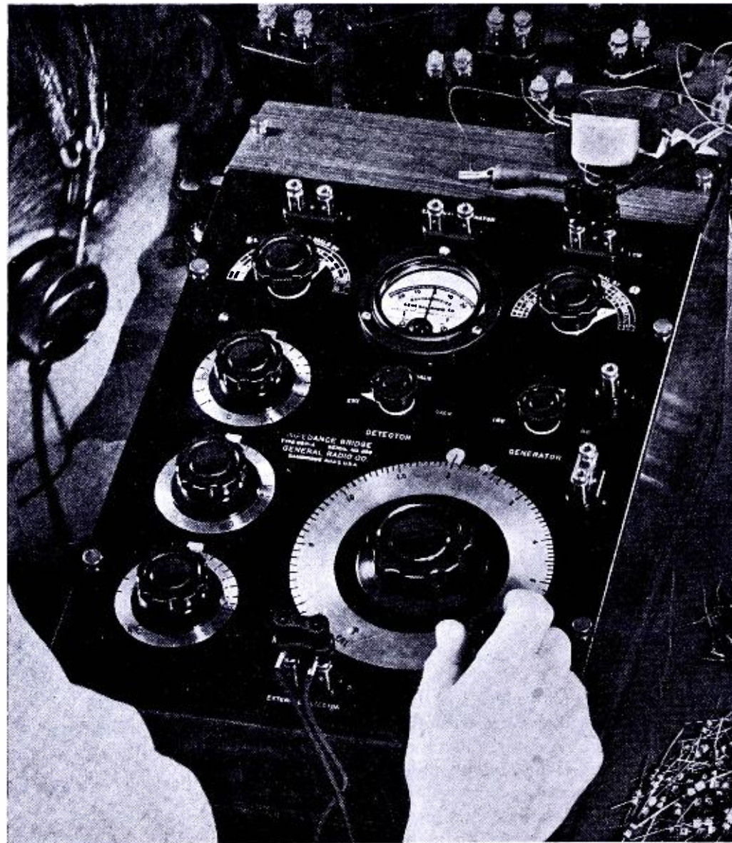
Figure 3 A typical impedance bridge, with Wheatstone bridge circuit. (Courtesy General Rad
