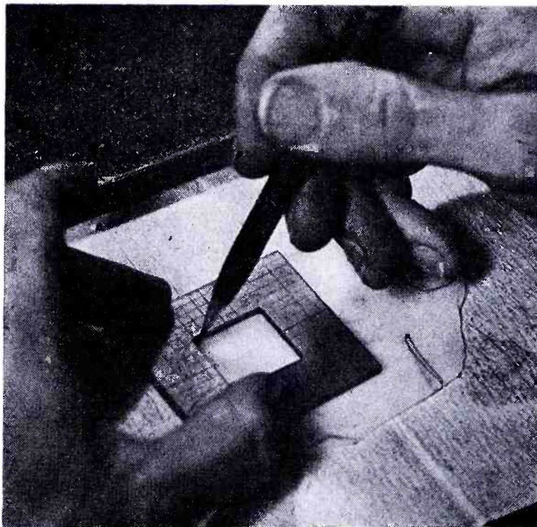
Figure 5 Layout jig used to draw the outlines for dicing or trim sawing. One edge of the blank is parallel to the X-axis. Note the marked spot on the lower right hand side which locates a crack to be avoided in layout.
