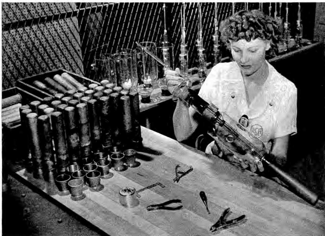
Much of the material extracted from tubes requiring rebuilding, can be reclaimed. Above we see quite a collection of such pieces, that have gone through the necessary processes that make them suitable for reuse.
