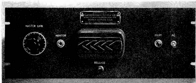
Front view of the alert device, showing the alarm bell in center.
