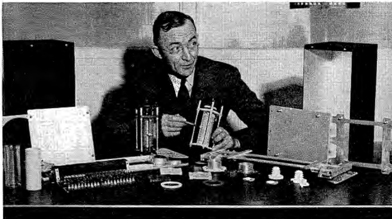
A few of the many components for which alternates have been designed at General Electric. Mr. Farrell is shown with a tuning inductance in which mycalex has been substituted for steatite and aluminum.
