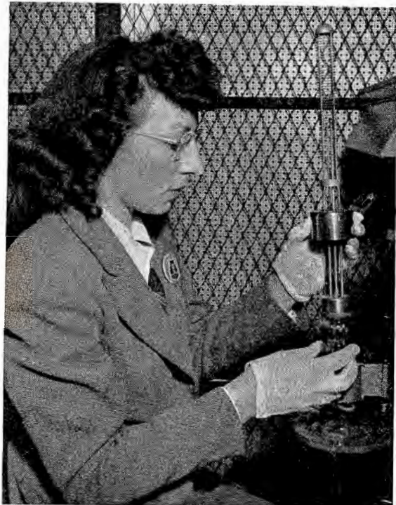
Assembling a new filament, and other internal parts as required, so that the tubes may meet standard requirements.
