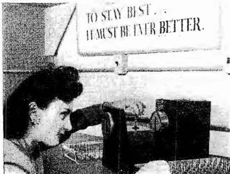
Bead tester utilizes polarized light in search for stress points in glass beads which seal leads to bulbs
