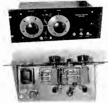
Front and interior views of the specially developed frequency measuring oscillator that affords an unusual degree of accuracy for direct measurement.
