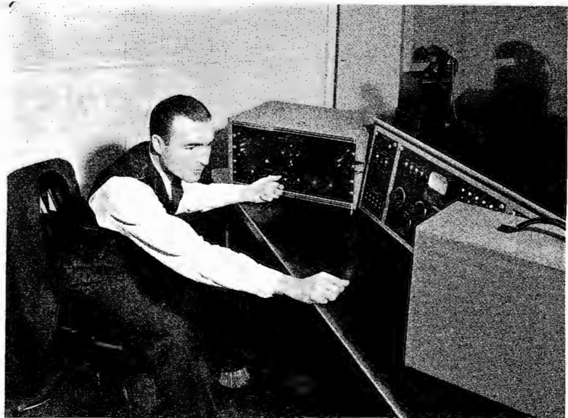
A square wave generator (left) being used to check studio speech input equipment. At right is a cathode-ray oscilloscope used to check the shape of the square wave after it has passed through the speech input equipment.
