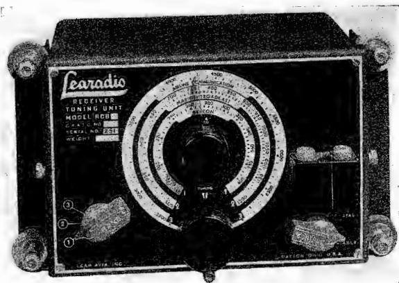
Figure 6 The model RCBB receiver that employs a calibrated dial prepared by the exact mathematical methods described here.
