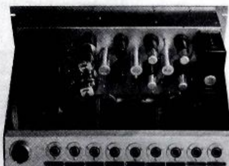
Fig. 11. (Above) Back view of amplifier showing physical layout.
