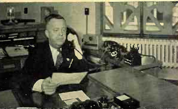
Fig. 16. An unusual intercommunication installation by Morlen Electric Co. in the Metropolitan Life Insurance Co.'s main offices links five executives' desk sets with 10 talk-back speakers in the supply department, the latter so sensitive to pick-up that supply clerks can talk back from any point without interrupting their work.
