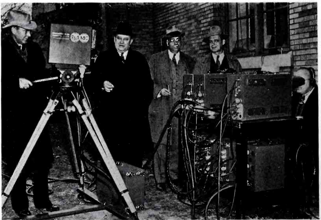
FCC members see new RCA television field equipment. Left to right: James Lawrence Fly, Thad. H. Brown, Norman S. Case, T. A. M. Craven. This portable equipment, developed by RCA engineers, is assembled in carrying cases weighing from 35 to 72 pounds.
