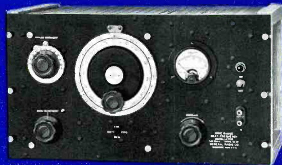
Left to Right: Type 700-A Beat-Frequency Oscillator, 50-cycle frequency meter—output potentiometer, 2500 Hz, low calibration—range control, zero beat control.
