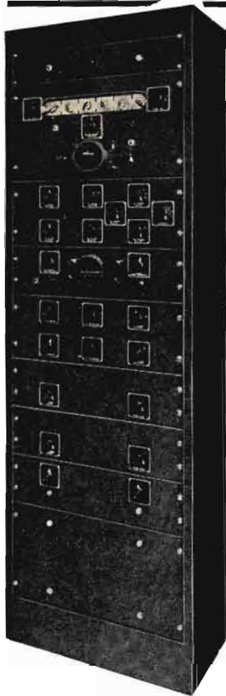
Type 203 Synchronizing-Signal Generator furnishes outputs as follows: Horizontal and Vertical Blanking Signals; Horizontal and Vertical Synchronizing Signals; Vertical Equalizing Pulses; Linear Horizontal Sweep Wave; Linear Vertical Sweep Wave; Special Sharp Vertical Synchronizing Pulses; and Special Horizontal Pulses.
