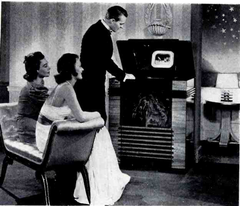
RCA Model TRK-12. Indirect viewing 12" kinescope, picture 7 3/8" x 9 3/4". Electric tuning for sound reception is provided for 9 stations.
