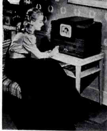
RCA television attachment TT-5. Utilizes chassis and speaker of any a-c radio for sound. Plugs into jack on 1938-39 RCA radios. Uses 5-inch kinescope.
