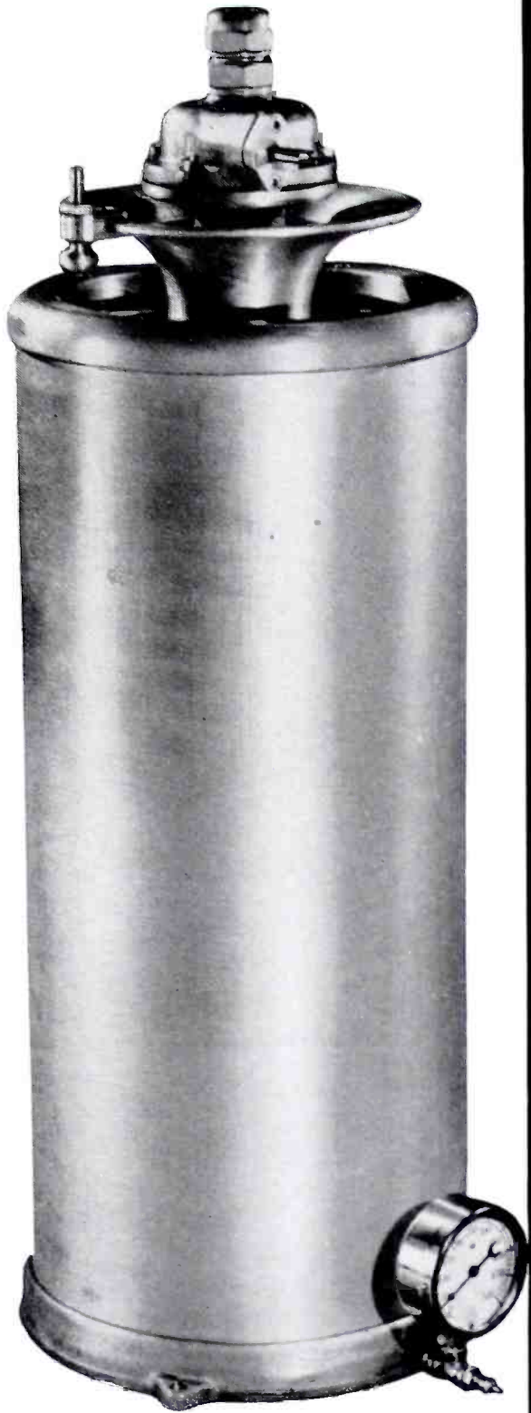
Lapp variable condenser Y150V15 100 amp., 15 KV (carrier RMS, 100% modulation) Capacitance 600-1500 mmf. External dimensions: Height, 34"; diameter, 11"
