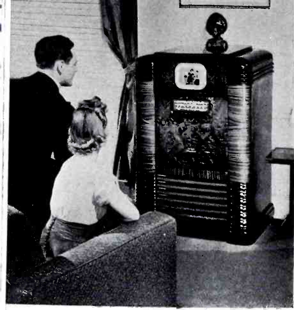
RCA's Model TRK-9. 9" kinescope, images 5 1/2" x 7 1/4", includes 12-tube, 3-band radio and switch for victrola attachment. Model TRK-5 (not shown) has 5" tube and 8-tube all-wave radio.
