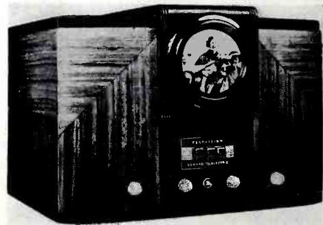
Right: G. E. HM-171 picture receiver and sound converter. 5" tube. Can be used with special receivers to be announced, or for pictures only.
